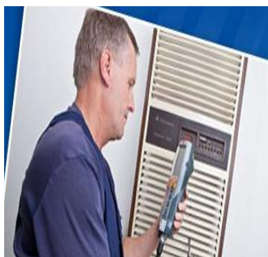
TESTING A GAS HEATER WITH A CARBON MONOXIDE ANALYSER
